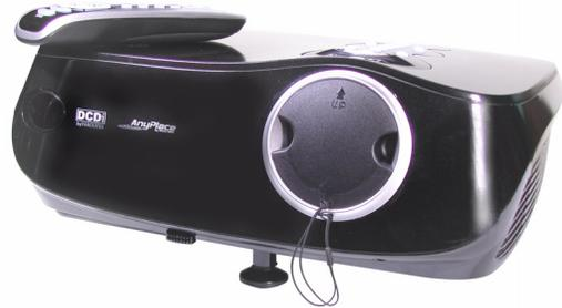
The projector is equipped with a full set of I/O connectors, enabling you to attach a wide variety of input devices including Composite Video, S-Video, Digital Video Interface (DVI), Computer VGA, and Component Video.
